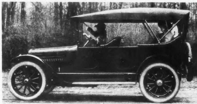
4. "Then you see I fasten it tight on the top of the windshield by turning the thumb screws. All done now. Simplest thing you ever saw."
